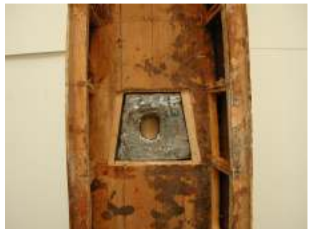
Forward ballast installed
